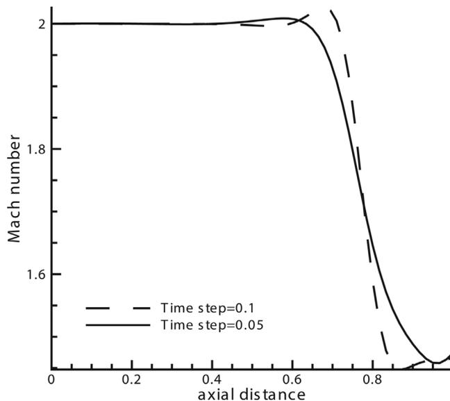
Figure 5. Mach number distribution at the centreline for different time steps for the OWF problem.
