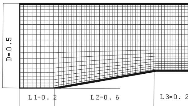
Figure 1. Geometry and grid for the OWF problem.
