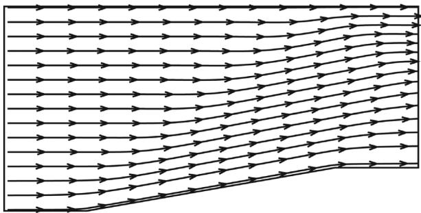
Figure 4. Redirecting the flow by shock wave, then by expansion fan, for the OWF problem.
