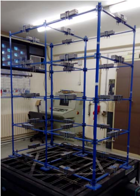
Figure 4. The reduced steel structure model.
