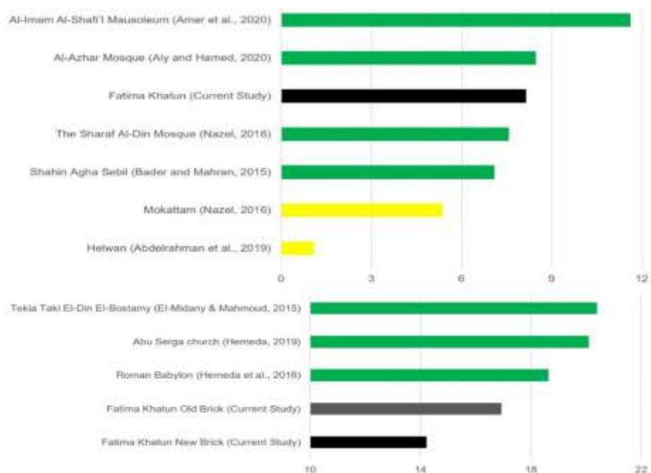
Fig. 12. Comparison of the water absorption (%) with the literature for the limestone (top) and the brick (bottom).
