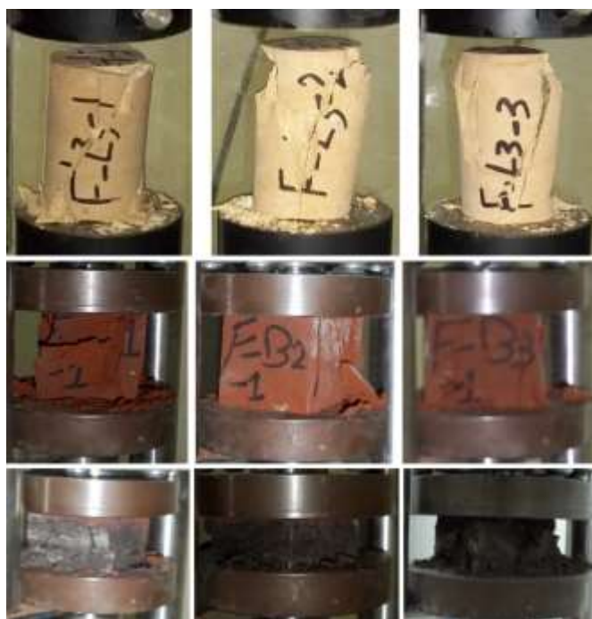
Fig. 14. Failure of the samples in the compressive strength test: The limestone (top), the new brick (bottom), and the old brick (bottom)
