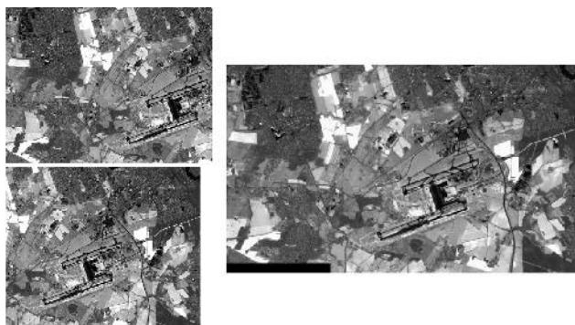
Figure 7. Two Rapid-Eye images for the area of Berlin Brandenburg airport (left) and their registered version (right) using SURF
