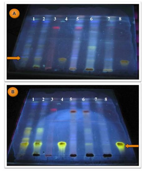
Figure 2: TLC of standard and sample solutions; *lane* 1: *in vivo* rhizome, *lane* 2: *in vitro* rhizomes, *lane* 3: *in vitro* shoots, *lane* 4: standard, *lane* 5: *in vitro* roots, *land* 6: *in vitro* microrhizomes, *lane* 7: callus cultures and *lane* 8: standard. A: after sprayed with 10% sulphuric acid and B: after heating. Plate: Silica gel 60  $F_{254}$  (20x20 cm). Solvent system: n-hexane–acetone (8:2).
