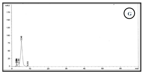
Figure 3: HPLC chromatogram showing the presence of 6-gingerol, A: synthetic standards, B: *in vivo* rhizome C: *in vitro* rhizomes, D: *in vitro* shoots, E: *in vitro* roots, F: *in vitro* microrhizomes and G: calli cultures.
