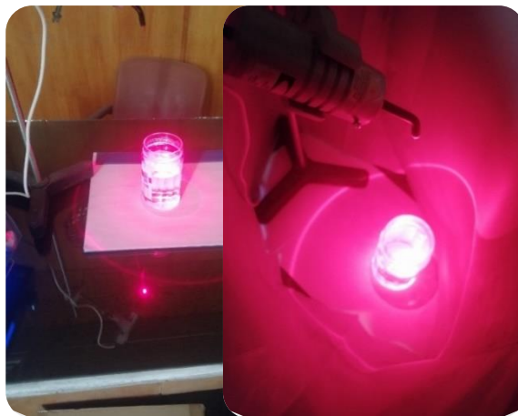
Fig (1) Photo of samples with laser irradiation (diode laser)
