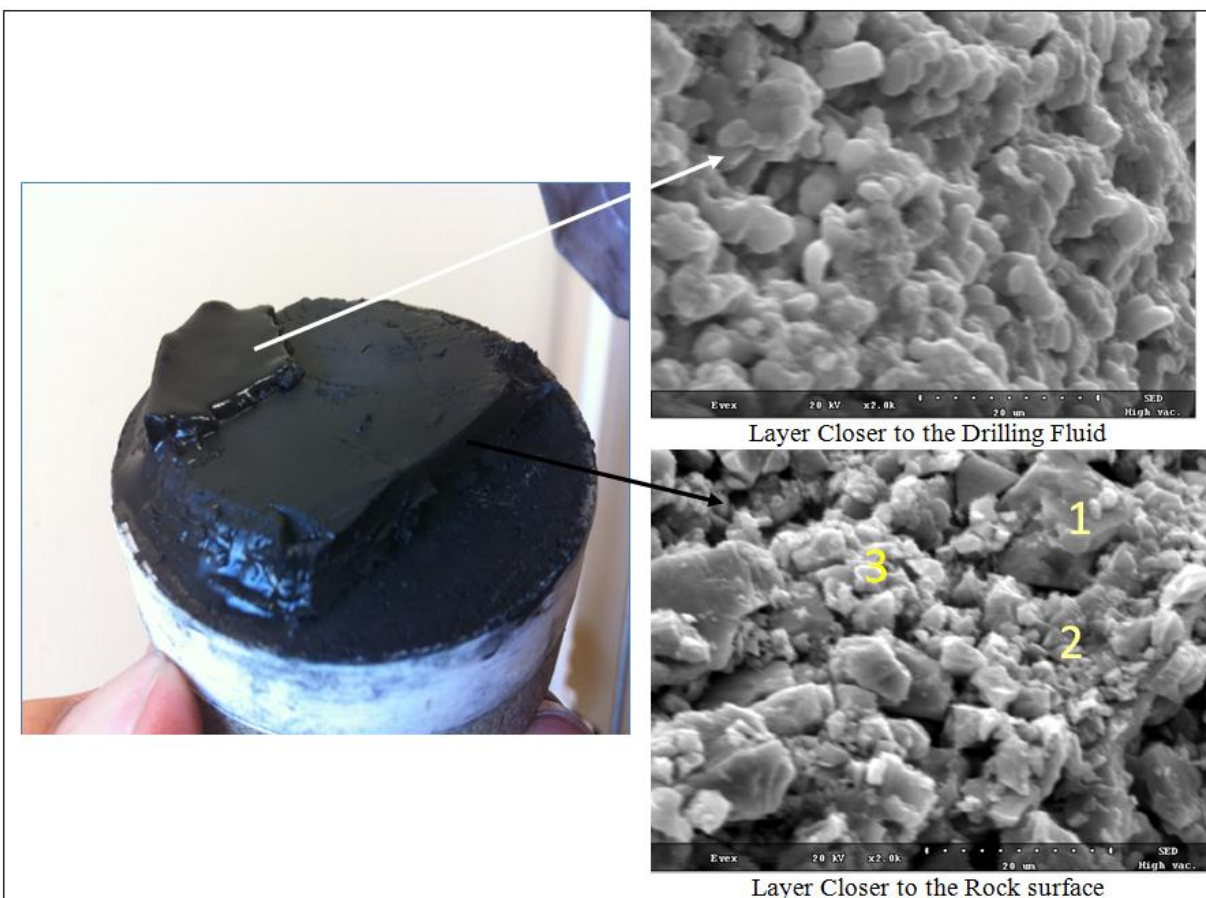
Fig. 14: SEM analysis shows the heterogeneity of the filter cake.
