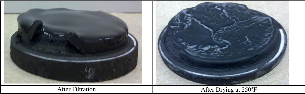
Fig. 7: 0.22 in. filter cake when using 400 g ilmenite.
