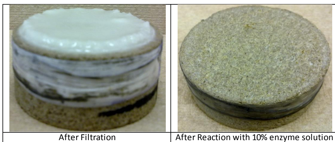
Fig. 13: Completely removal of the filter cake using the ratio of \text{CaCO}_3 to PLA 1:3.
