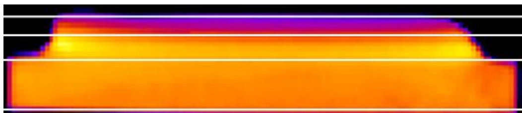
Fig. 6: Filter cake layers of the drilling fluid drilling fluid C with 10.3 ppg.
