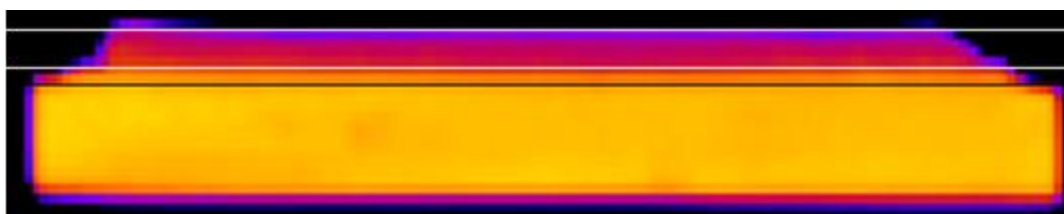
Fig. 5: Filter cake layers of the drilling fluid of 9.6 ppg.
