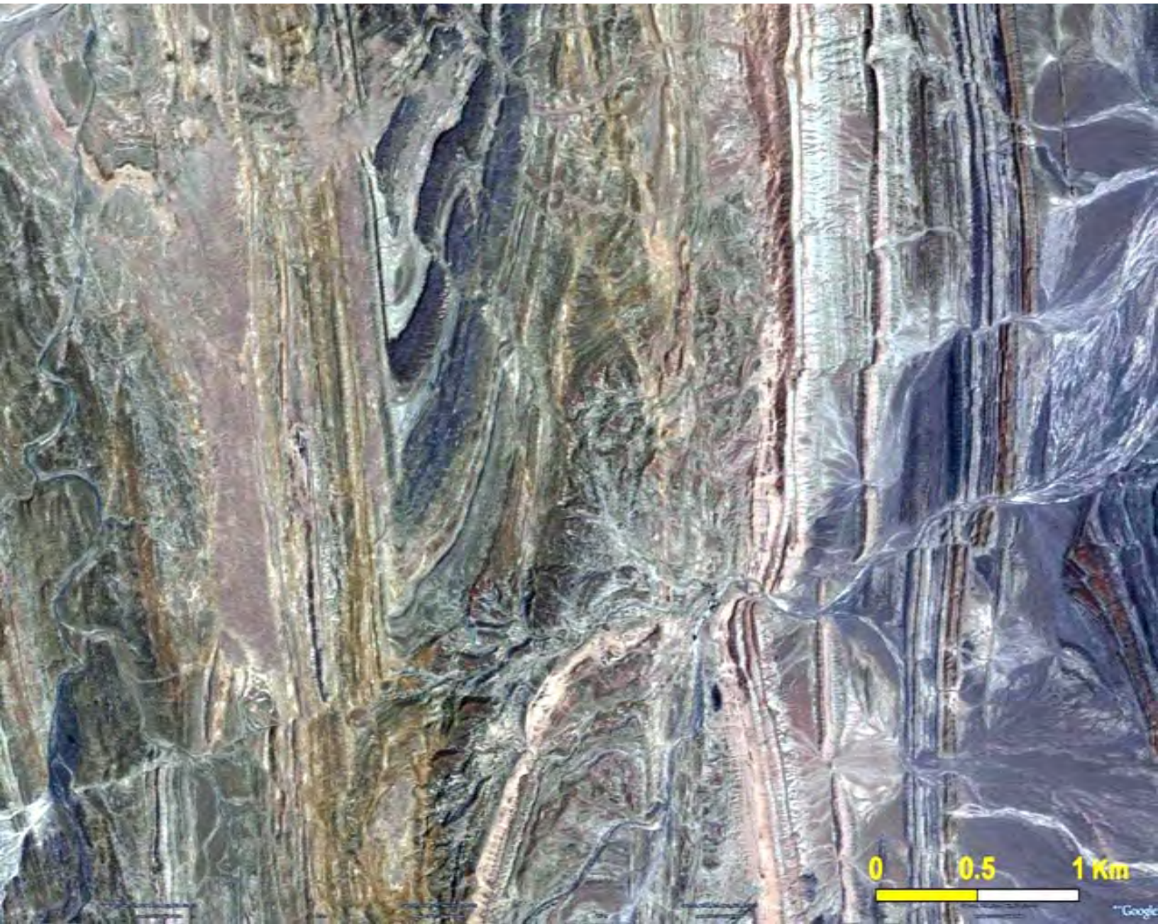
Master and minor faults. Jurassic, Iran Notice the dragging of bedding along the master fault.
