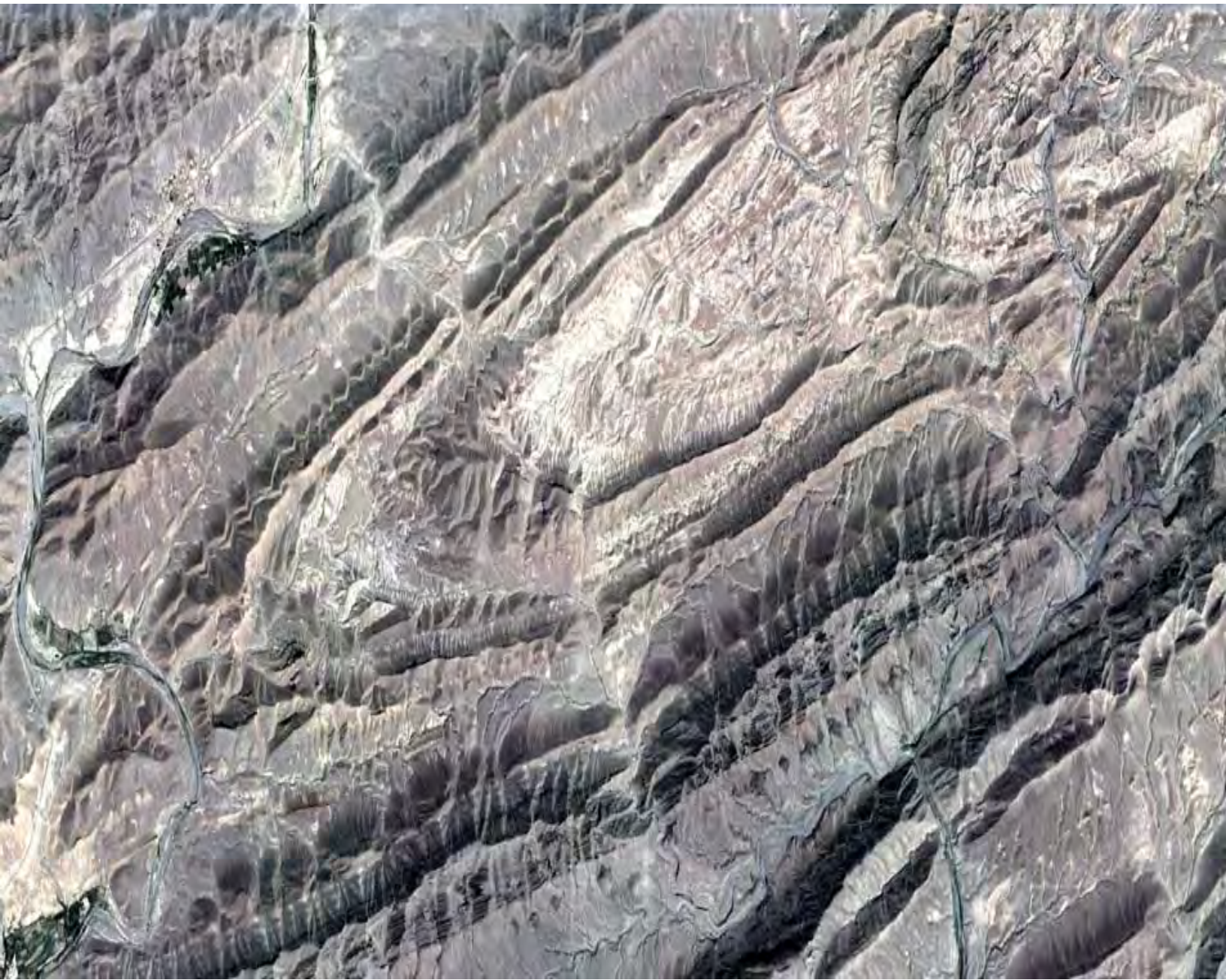
Anticlinal Fold in sedimentary succession. Notice, the direction of plunge to the SW, and the V shapes in the northern limb. Width of the image= 5 Km.
