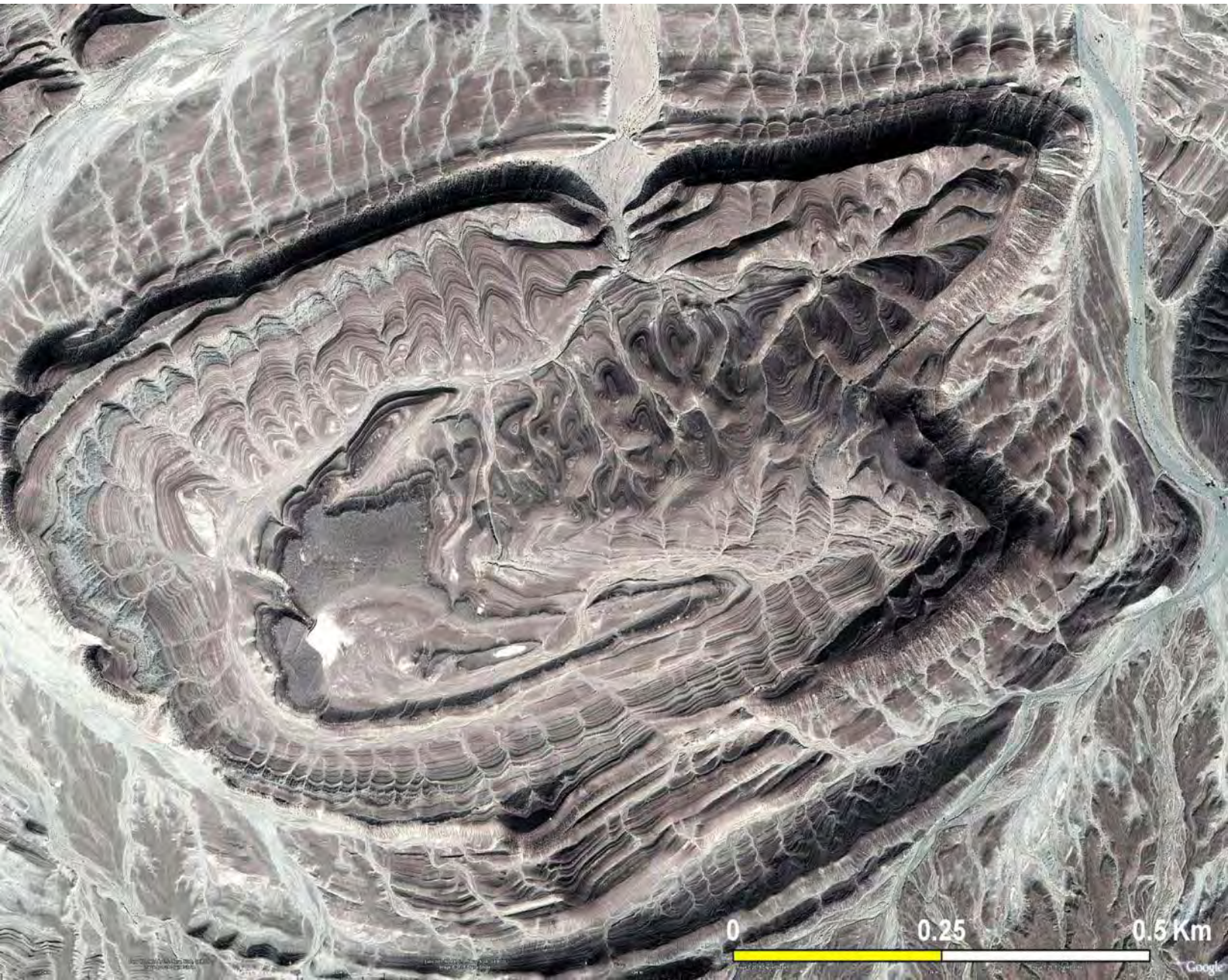
Complex folding in Cenozoic sedimentary rocks, Pakistan. Notice, the V shapes in bedding inside the structure, indicating a basin structure.
