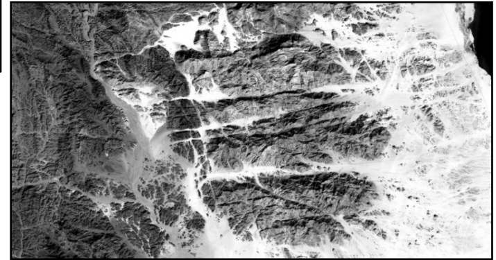
Landsat image. DN values represent brightness of each pixel
