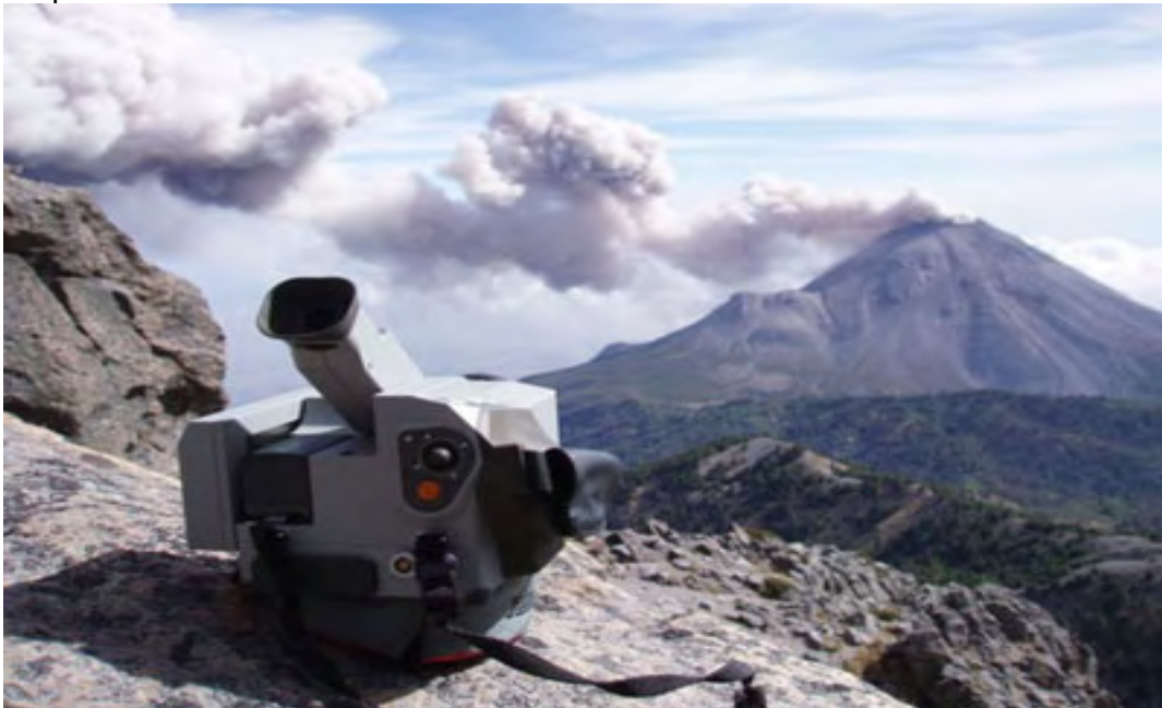
Figure 1: Example of a thermal radiometer measuring radiant flux of an emitting object. Source: http://www.ucol.mx/ciiv/geochem/thermal_en.htm In general, thermal radiometers, which measure the objects radiant temperature can be used as a proxy for the objects true kinetic temperature.
