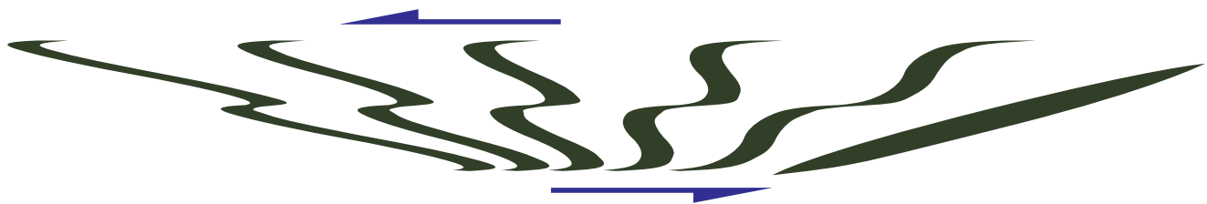
Figure 15.31 Progressive development of folds in simple shear (strain increasing to the left). This particular initial orientation can result in a vergence apparently inconsistent with the sense of shear.
