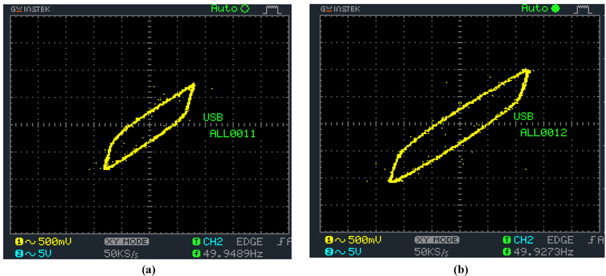
Figure 10 Lissajous figures of DBD reactor using argon gas (flow rate 3 L/min) at applied voltages V_{pp} : (a) 18 kV and (b) 24 kV, respectively (X-axis \times 1.675 \mu\text{F} and Y axis \times 5 \text{ kV} )
