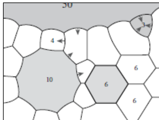
Fig 3.33: Boundary motion causing grain growth or shrinkage
