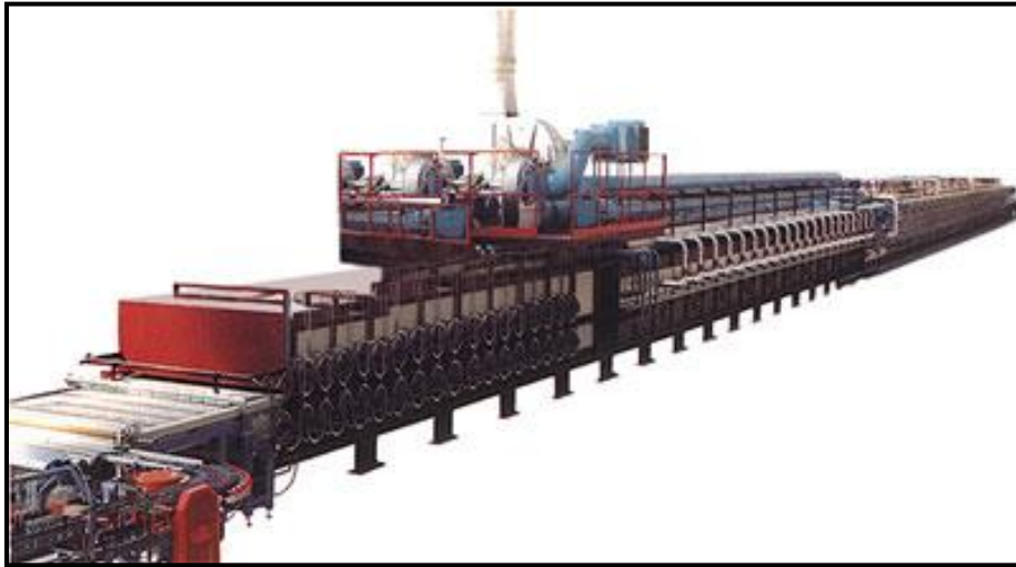
Fig 3.42: Photo of a roller kiln
