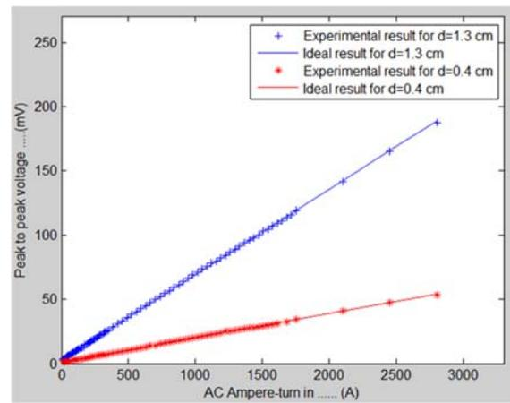
**Fig. 9.** The Peak to peak output voltage as a function of the applied AC current ( $I=Ni$ ) in the cases of  $d=0.4$  and  $1.3$  cm.
