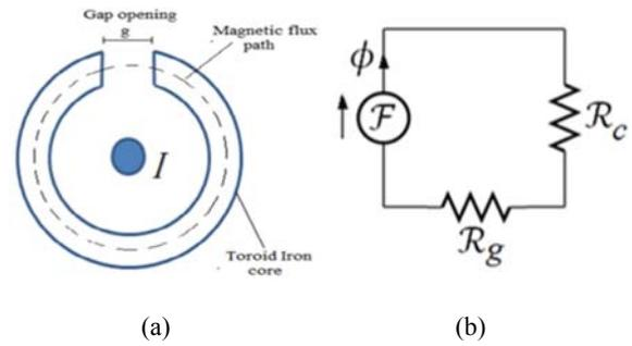
**Fig. 1.** (a) Toroid core with an air gap and (b) its electric representation circuit.
