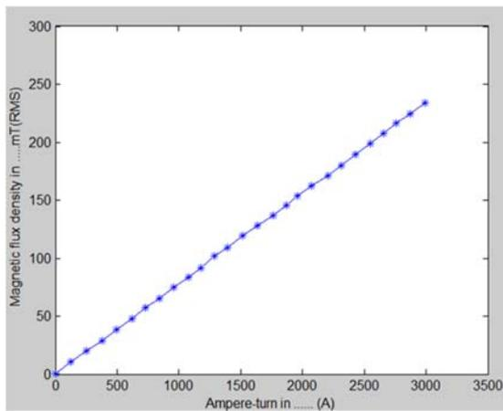
**Fig. 8.** The Ampere-turn versus the magnetic field in the gap center of the Toroid iron core.
