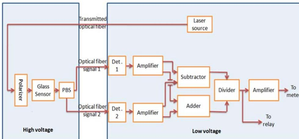
Fig. 3. Schematic block diagram of the proposed optical current transformer.
