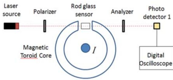
Fig. 2. The Dual quadrature Polarimetric schematic setup.
