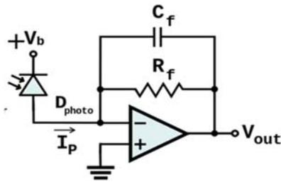
Fig. 4. The Transimpedance amplifier circuit.
