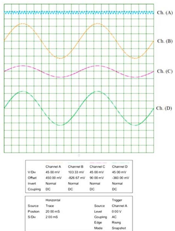
**Fig. 7.** Oscilloscope output - Ch. (A): Adder O/P signal, Ch. (B): Subtractor O/P signal, Ch. (C): Divider O/P current signal and Ch. (D): Amplified current signal.
