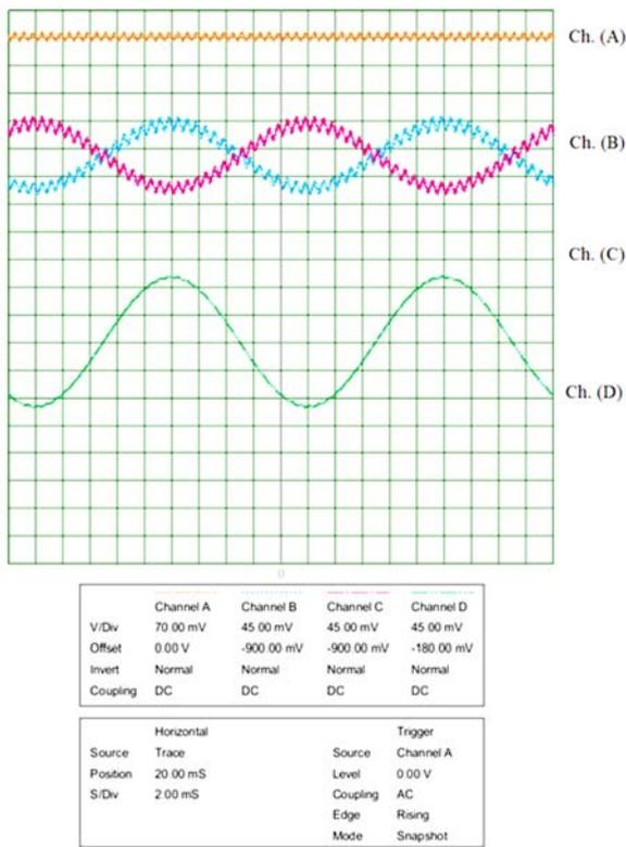
**Fig. 6.** Oscilloscope output - Ch. (A): light signal, Ch. (B): detector 1 signal, Ch. (C): detector 2 signal and Ch. (D): Subtractor O/P signal.
