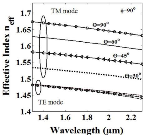
**Fig. 5** Variation of the birefringence with the wavelength at different tilt angles  $\Theta$  of the NLC director,  $0^\circ$ ,  $30^\circ$ ,  $45^\circ$ ,  $60^\circ$ , and  $90^\circ$
