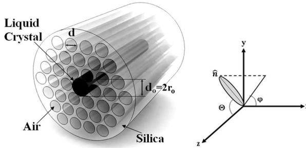
**Fig. 1** The structure of the suggested NLC-PCF. The tilt  $\Theta$  and twist  $\varphi$  angle definitions for NLC director are shown at the *right*
