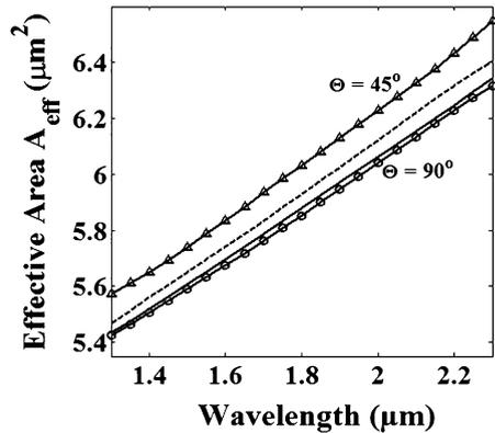
$45^\circ$  to  $90^\circ$ , the index contrast between the core and cladding region is increased. Therefore, the confinement through the core region increases. Consequently, the  $A_{\text{eff}}$  of the quasi TM mode decreases by increasing  $\Theta$  as shown in Fig. 5. For example, at  $\Theta = 45^\circ$ , and  $90^\circ$ , the  $A_{\text{eff}}$  equals to  $5.787$ , and  $5.633 \mu\text{m}^2$ , respectively at the operating wavelength  $\lambda = 1.55 \mu\text{m}$  as shown in Fig. 6.
