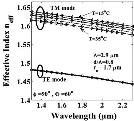
**Fig. 3** Variation of the birefringence with the wavelength at different temperatures, from 15 to 35  $^\circ\text{C}$  with a step of 5  $^\circ\text{C}$
