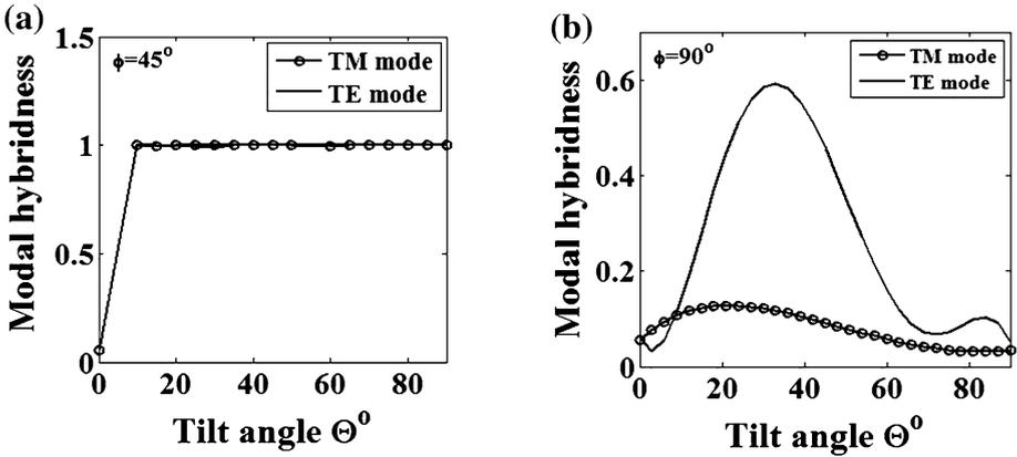
**Fig. 14** Variation of the modal hybridness of the two polarized modes with the tilt angle at the operating wavelength  $\lambda = 1.55 \mu\text{m}$  at **a**  $\phi = 45^\circ$ , **b**  $\phi = 90^\circ$
