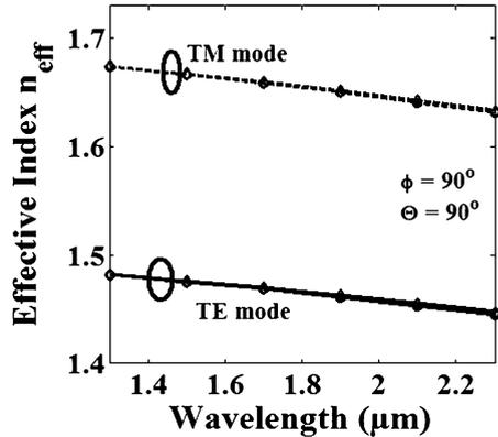
**Fig. 9** Variation of the birefringence with the wavelength at different core radii,  $r_o = 1.7, 1.6,$  and  $1.5 \mu\text{m}$
