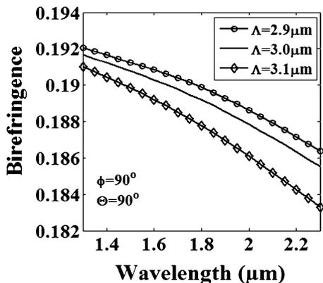
**Fig. 8** Variation of the  $n_{\text{eff}}$  of the two polarized modes with the wavelength at different hole pitches 2.9, 3.0, and 3.1  $\mu\text{m}$
