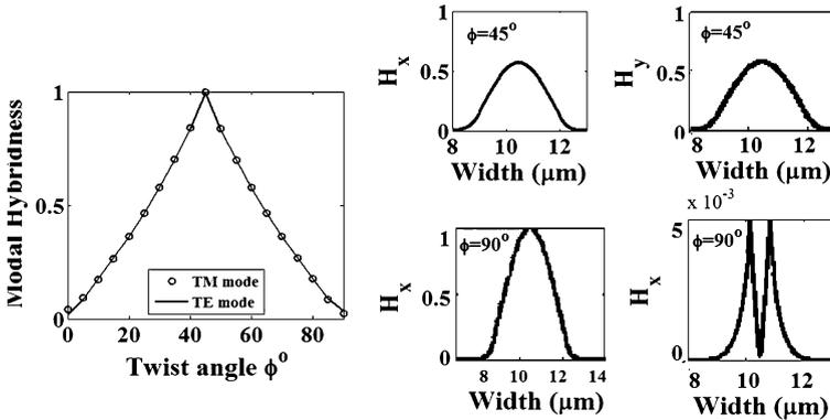
**Fig. 13** Variation of the modal hybridness of the two polarized modes with the twist angle at the operating wavelength  $\lambda = 1.55 \mu\text{m}$
