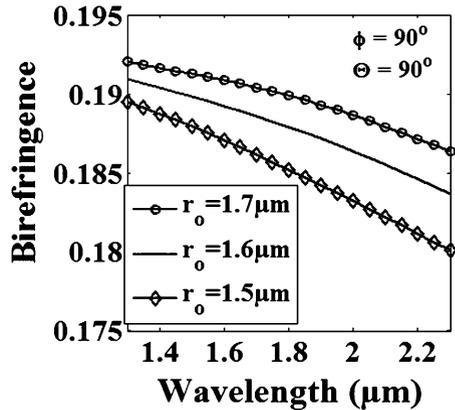
of the NLC infiltration increases. Consequently, the asymmetry of the structure and hence the birefringence increase. At NLC core radius  $r_o = 1.5, 1.6$  and  $1.7 \mu\text{m}$  the birefringence equals to 0.1875, 0.1895, and 0.1911, respectively at the operating wavelength  $\lambda = 1.55 \mu\text{m}$ .
