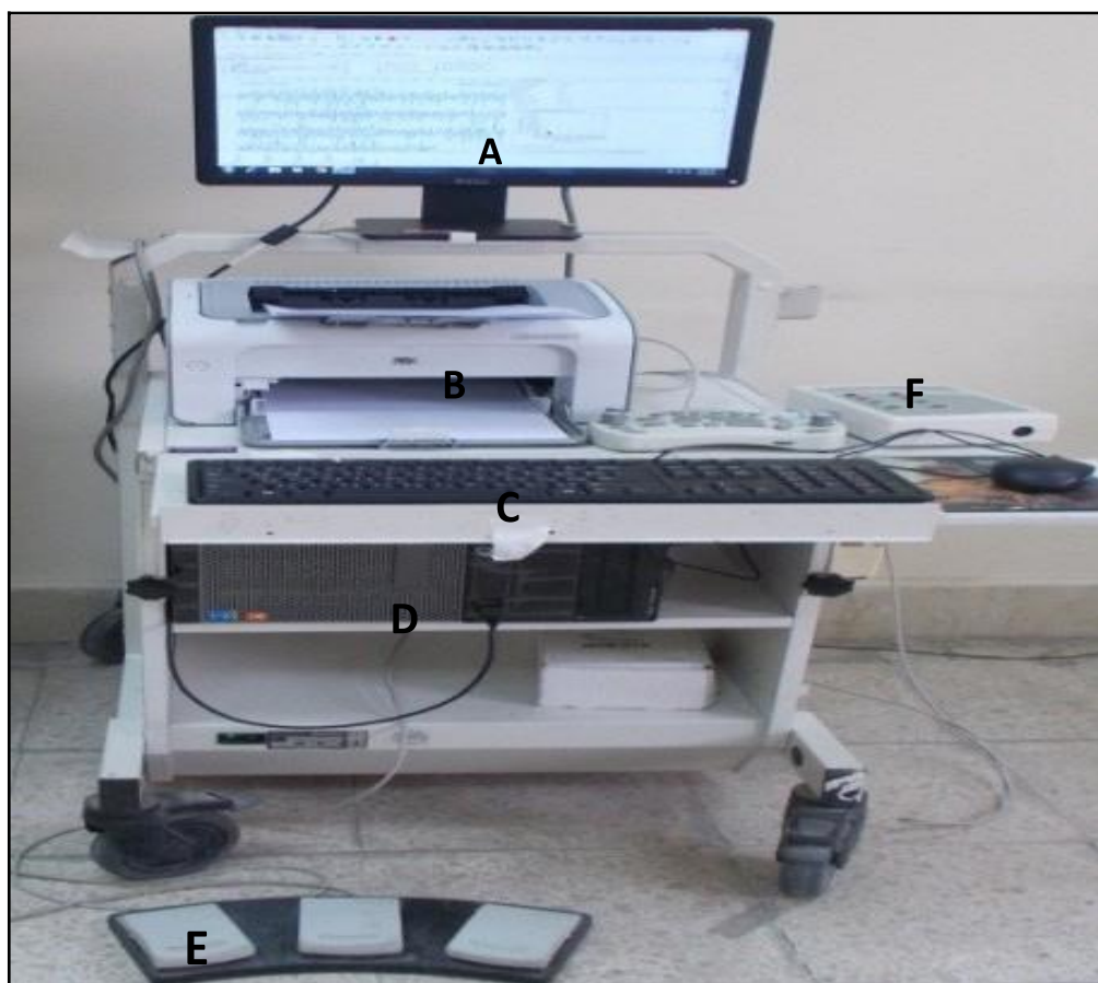
Figure (1): Surface electromyography system: (A) Screen, (B) printer, (C) key board, (D)Computer Processing unit, (E) Foot presser, (F) Amplifier. ( Patel, Anup.2015 )
