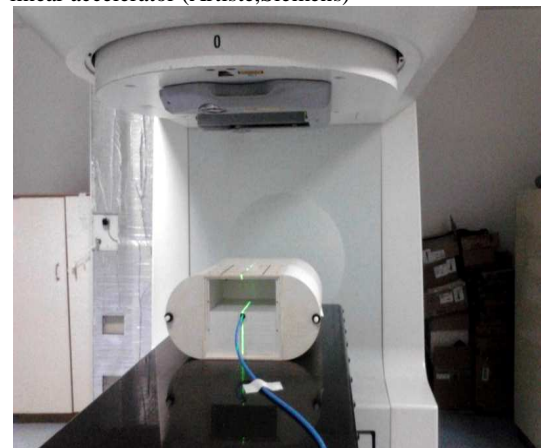
Figure 2: The EasyBody phantom measurements by the linear accelerator (Artiste, Siemens)
