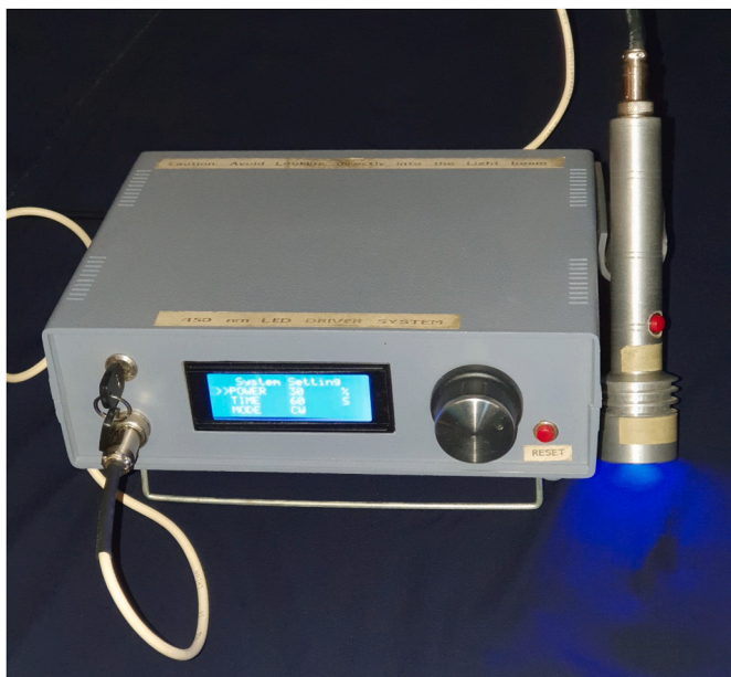
Fig. 1. light-emitting diode (LED) system, 450 nm, and 3 cm spot size.
